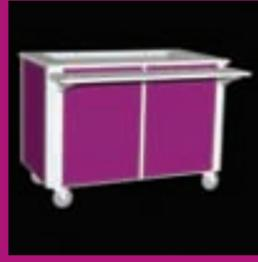
This all-in-one cooling unit makes remote service a breeze. Features a self-contained condensing unit with adjustable temperature control. Stainless steel cold pan is 7" deep and equipped with a 1" I.P.S. drain for easy draining and cleaning. Refrigeration tubing is attached to the sides of the cold pan and fully insulated with foamed-in-place polyurethane for better efficiency.
