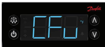
6. **-F** should be displayed indicating Fahrenheit. Use the down arrow to change it to **-C** for Celsius and hit the stand-by button (lower left button) to enter the change.
