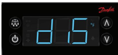
5. Scroll to **CFu** using the up/down arrows and push the stand-by button (lower left button) to enter the display unit menu.
