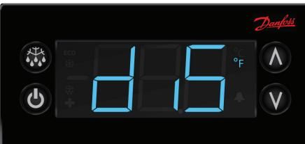
8. Push the defrost button (upper left button) to move out of the display menu and back to the normal display.
