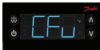
6.  $-\text{F}$  should be displayed indicating Fahrenheit. Use the down arrow to change it to  $-\text{C}$  for Celsius and hit the stand-by button (lower left button) to enter the change.
