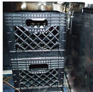
Correct location: 2" gap between crates and wall allowing proper air flow around crates.
