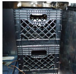
Incorrect location: Crates are too close to the wall and covering the fan, restricting air flow.
