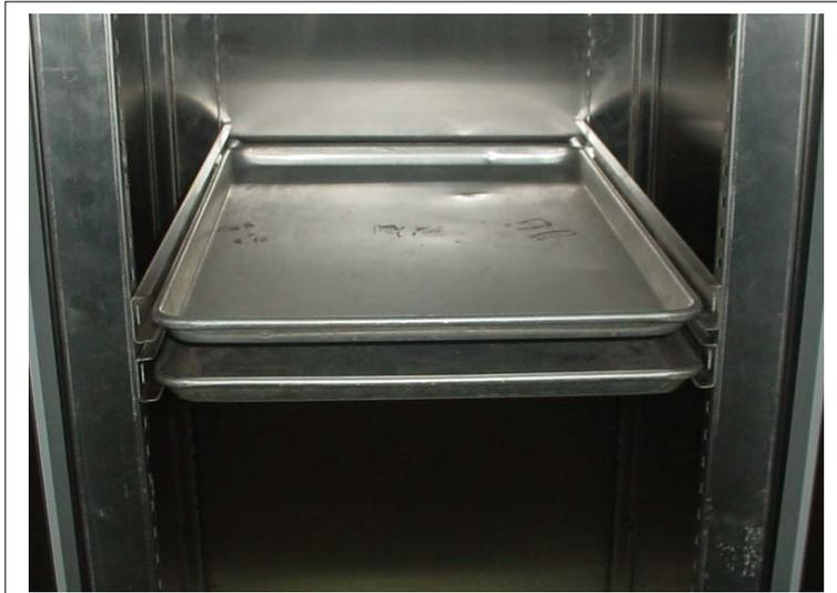
**3.1-1 – Installed T-1 Tray Slide with 18”x 26” Pans**
