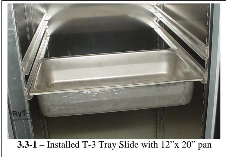
3.3-1 – Installed T-3 Tray Slide with 12”x 20” pan
